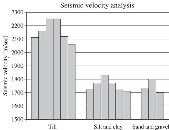
Fig. 6. Velocities calculated from VSP in five exploratory drillings penetrating the sediment fill in buried valleys of Vejle County. Two distinct velocity groups appear: Clay/silt and sand/gravel at  $1750 \pm 100$  m/s, and till at  $2150 \pm 100$  m/s.
