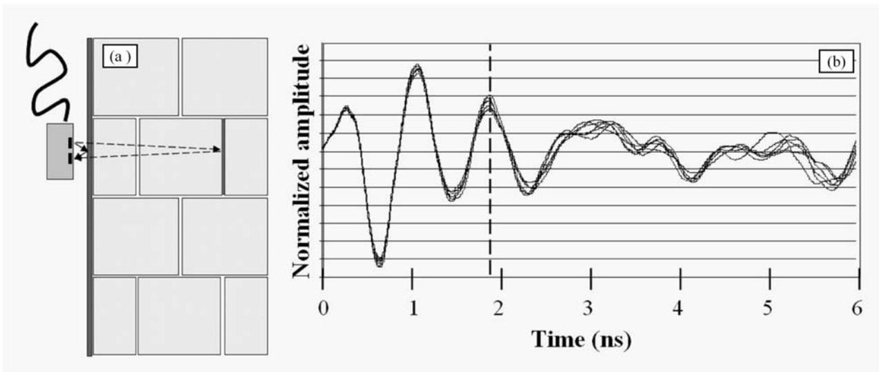
**Figure 9.** (a) Sketch of a typical GPR acquisition along the surface of a wall using semi-transparency techniques; (b) traces of GPR signals showing the shape of the first arrivals (first part, up to the vertical broken line) and that of later arrivals (about 2 ns delay). The ways of the latter waves, in the presence of an external patina, cross the patina layer twice (after Cosentino and Deganello, 2003).
