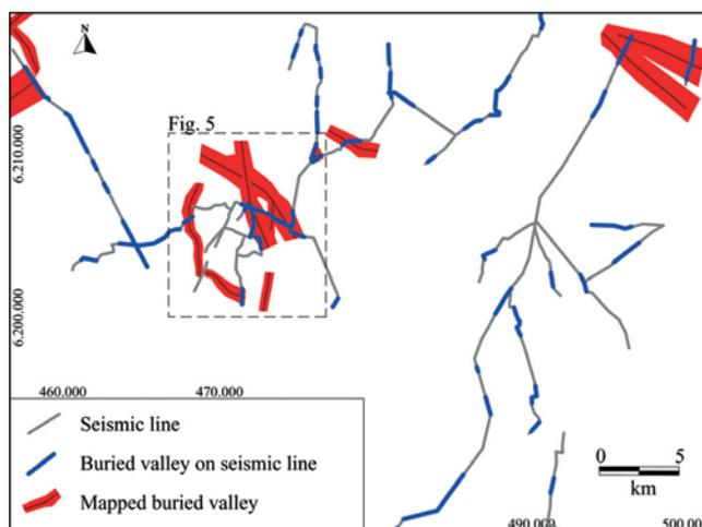
Fig. 7: A selected area in the western part of Jutland showing the high frequency of buried valleys found in seismic data. Correlations between the seismic lines require dense geophysical data grids. The Rækker Mølle area (Fig. 5) is marked. Coordinate system in metres (UTM zone 32/euref 89).
