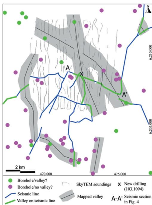
Fig. 5: A selected area with buried valleys in the western part of Jutland (Rækker Mølle area). The mapped valleys and the data used for the mapping of the valleys are shown. Coordinate system in metres (UTM zone 32/euref 89).
