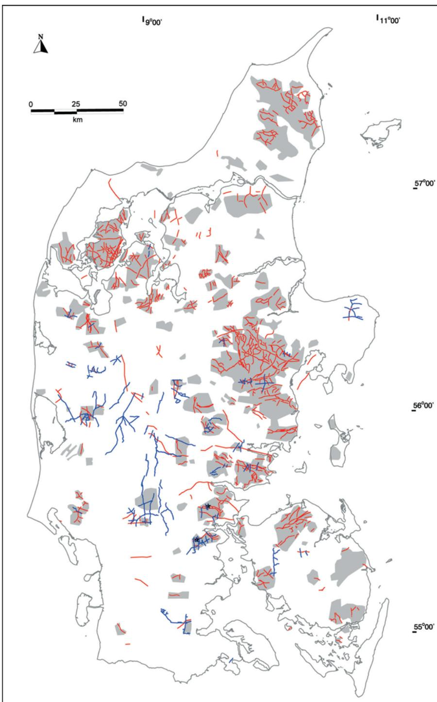
Fig. 6: Mapped buried valleys, TEM surveyed areas and high-resolution seismic sections in Jutland and Funen. Mapped buried valleys shown with red lines, seismic sections with blue lines and TEM surveyed areas in grey.
