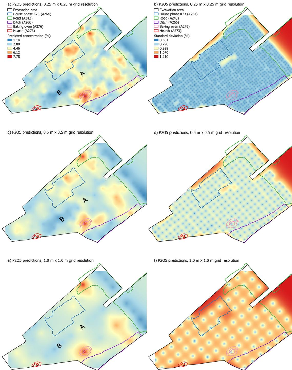
**Fig. 6** Predicted surface elemental concentrations and variance on the predictions for  $P_2O_5$  in the 0.25-m  $\times$  0.25-m grid (a and b), 0.5-m  $\times$  0.5-m grid (c and d), and 1.0-m  $\times$  1.0-m grid (e and f)
