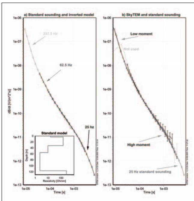
Fig. 5. The Lyngby standard sounding is made using the PROTEM47 system in a 40 × 40 m<sup>2</sup> central-loop configuration. (a) The three curves correspond to repetition base frequencies of 237.5 Hz, 62.5 Hz, and 25 Hz, and transmitter currents of 1, 3, and 3 A, respectively. The model is the corresponding 1D inversion result. (b) The comparable SkyTEM sounding in static mode using the same configuration as for (a).
