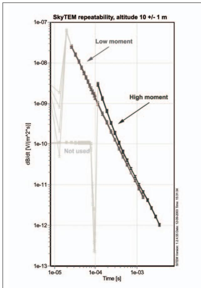
Fig. 8. Data from a base station for a survey south of Aarhus. The sounding was repeated four times within a day. Deviations of less than 5% are due to variations of  $\pm 1$  m in flight height from the nominal altitude of 10 m.
