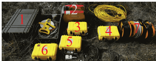
Figure 7. The Apsu system. (1) ApsuPS, (2) generator, (3) ApsuTx, (4–6) ApsuRx, and (7) transmitter and receiver coils. The photo also shows the communication and power cables.
