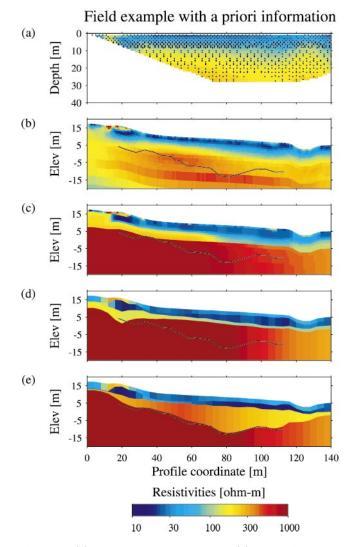
Figure 6. (a) The data pseudosection. (b) The minimumstructure L2 norm inversion result. (c) The corresponding L1 norm inversion result. (d) The 2D LCI result without a priori information. (e) Includes depth to the bedrock as a priori information. The depth to the bedrock from the refraction seismic data is drawn as a black line.
