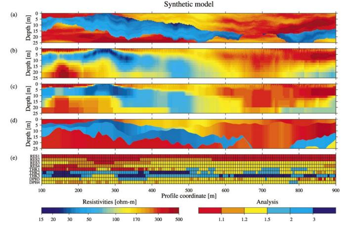
Figure 4. (a) The true model, with a clay layer of 30 ohm-m interbedded in a sandy layer of 300 ohm-m. (b) The minimum structure L2 norm inversion result. (c) The corresponding L1 norm inversion result. (d) The 2D LCI result. (e) An analysis of the model parameters (resistivities, RES1–RES4; thicknesses, THK1–THK3; and depths, DPH3-DPH4). The analysis uses a six-graded color code ranging from red (well determined) to blue (undetermined).
