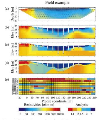
Figure 5. (a) The data pseudosection. (b) The minimum structure L2 norm inversion result. (c) The corresponding L1 norm inversion result. (d) The 2D LCI result with the parameter analyses in (e). The color-coding of the analyses ranges from well resolved (red) to poorly resolved (blue). Lithological logs from drillings are located every 20 m from coordinate 20 to 200 m. The colors of the drillholes indicate, from the bottom, rock (dark gray), till (light gray), and clay (white).
