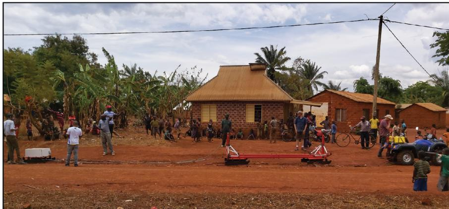
**Figure 1.** Picture of the tTEM system. The transmitter frame (red) is towed approximately 3.5 m behind the ATV, while the receiver coil (white box) is towed 7 m behind the transmitter. All instrumentation sits on the ATV, as well as a tablet streaming data and GPS location for data quality control and navigation.
