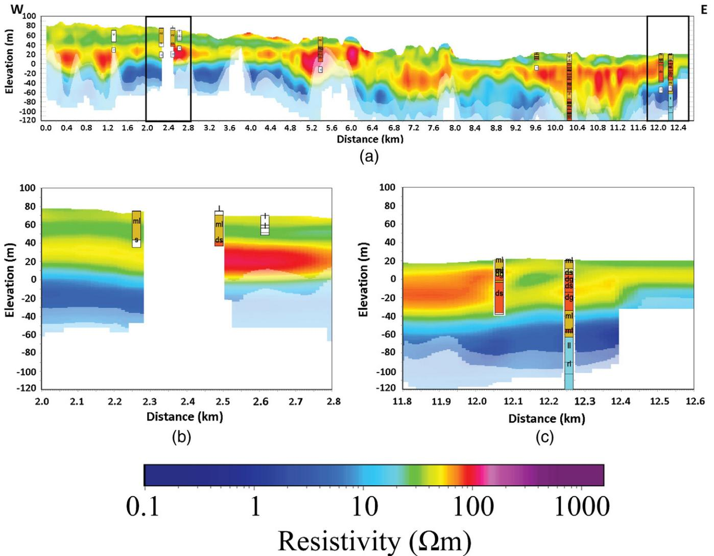
**Fig. 5.** SkyTEM results from the Norsminde catchment: (a) resistivity section of the profile drawn as a black line on map of Fig. 5 with borehole data; (b) zoom on the West part of the cross-section; (c) zoom on the East part of the cross-section. Borehole legend: dg = glacial gravel, s = sand, ds = diluvial sand, l = clay, ml = moraine clay, ll = plastic clay and rl = Eocene clay. All displayed boreholes are located within less than 50 m from the profile.
