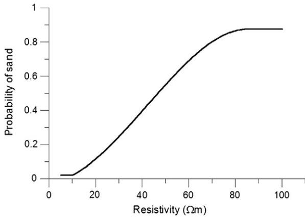
Fig. 6. Relationship between resistivity of SkyTEM soundings and probability of sand/clay in the Norsminde area for the best quality boreholes.
