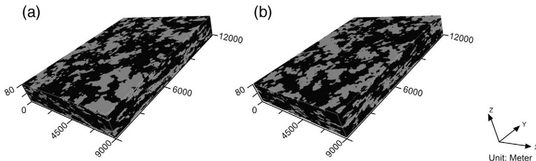
Fig. 7. Examples of two TProGS realisations from the Norsminde area. The dark and light colours correspond to clay and sand respectively.
