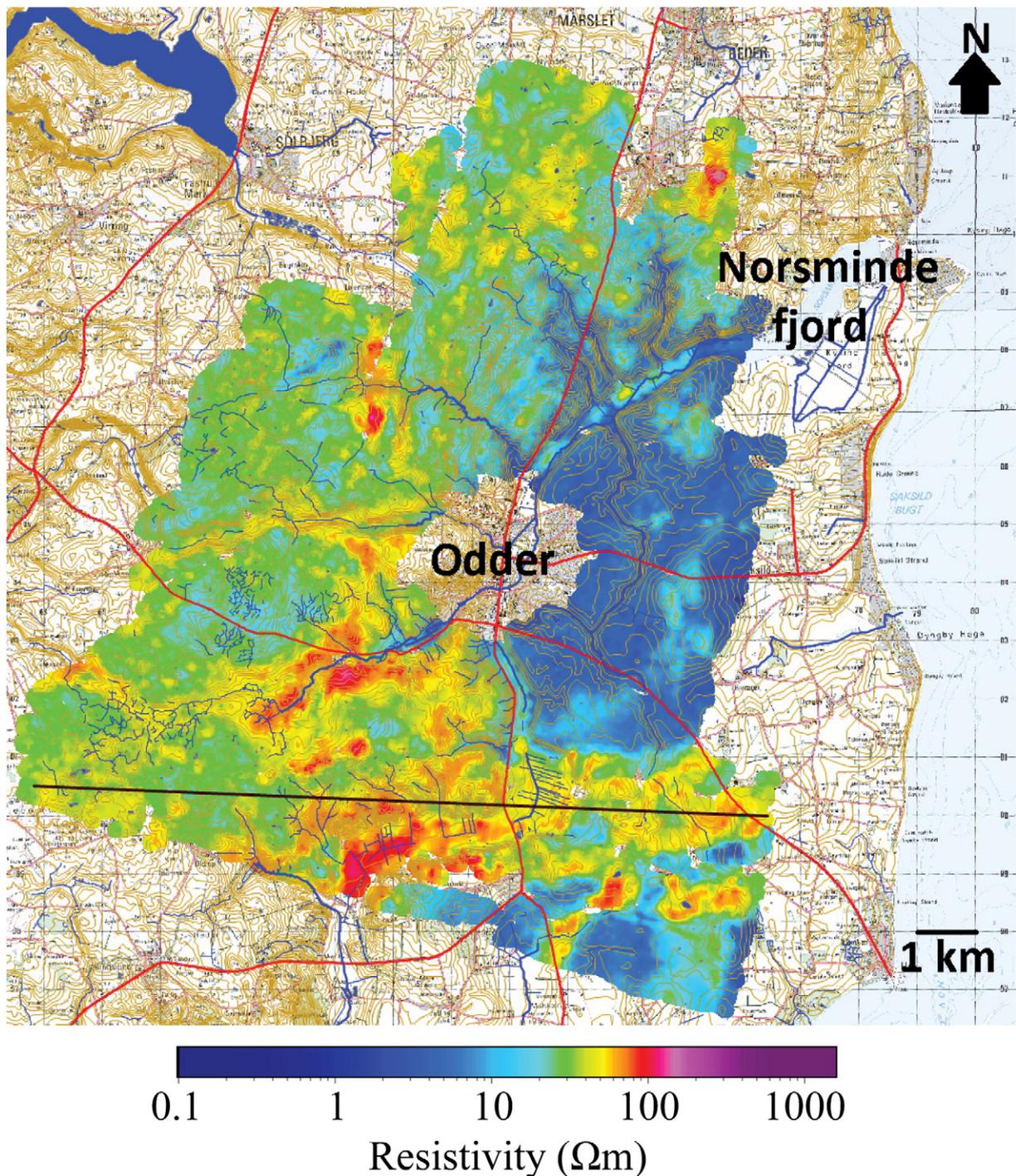
**Fig. 4.** SkyTEM results from the Norsminde catchment: Mean resistivity map of the depth interval 15–20 m. Results are obtained after a spatially constrained inversion with 29 layers from 1.5 m to 150 m depth. The map is obtained after kriging with a search radius of 150 m. Light brown lines correspond to topographical isolines, blue ones to streams, and red ones to main roads.
