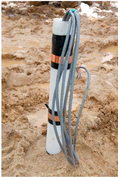
Fig. 2. Photo of the installed electrode-tube in B3, showing two unused electrodes above ground. The wires coming out, were connected to the instruments.
