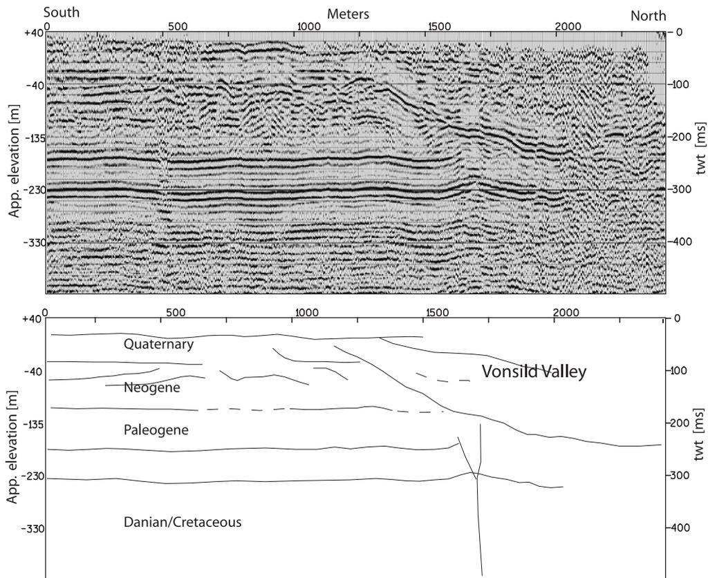
Fig. 7. The southern flank of the Vonsild valley shown on a reflection seismic section (unmigrated 32-fold stack). Interpretations sketched below the seismic section. Location of the seismic section is shown in Fig. 6 as a solid black line. Data collection and processing by Rambøll (Jensen et al., 2002).
