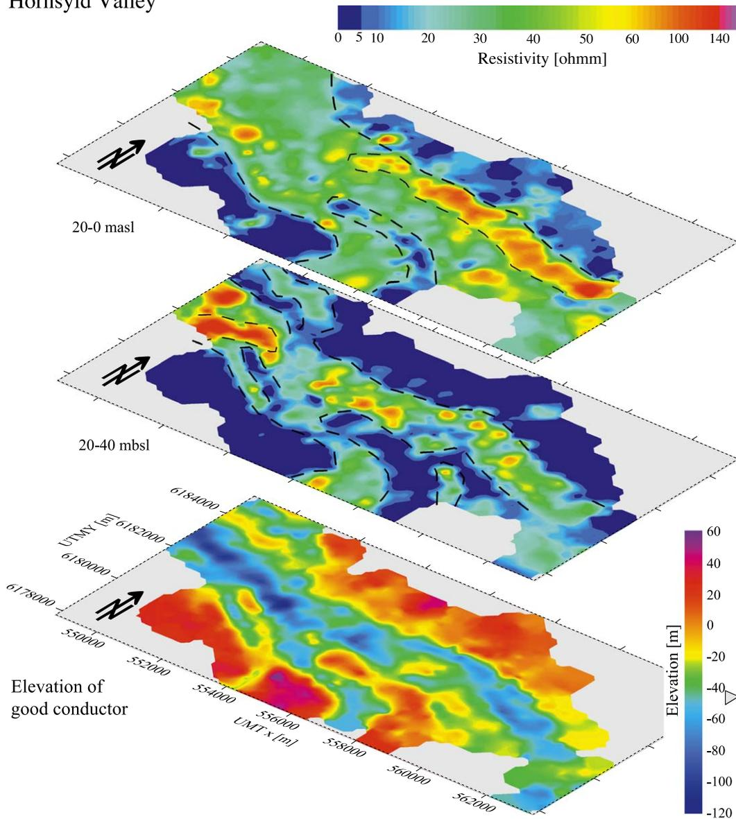
Fig. 3. Contour maps showing the buried Hornslyd valley. The valley is imaged on two depth slices of mean resistivity and on a map showing the elevation of the deepest good conductor as defined by resistivity values less than  $7 \Omega \text{ m}$ . The maps are based on 1-D inversion models of 734 TEM and HiTEM soundings. Thick dashed lines mark valley boundaries. Thin dashed lines mark internal incision boundaries. Field survey: Dansk Geofysik, Rambøll and WaterTech.
