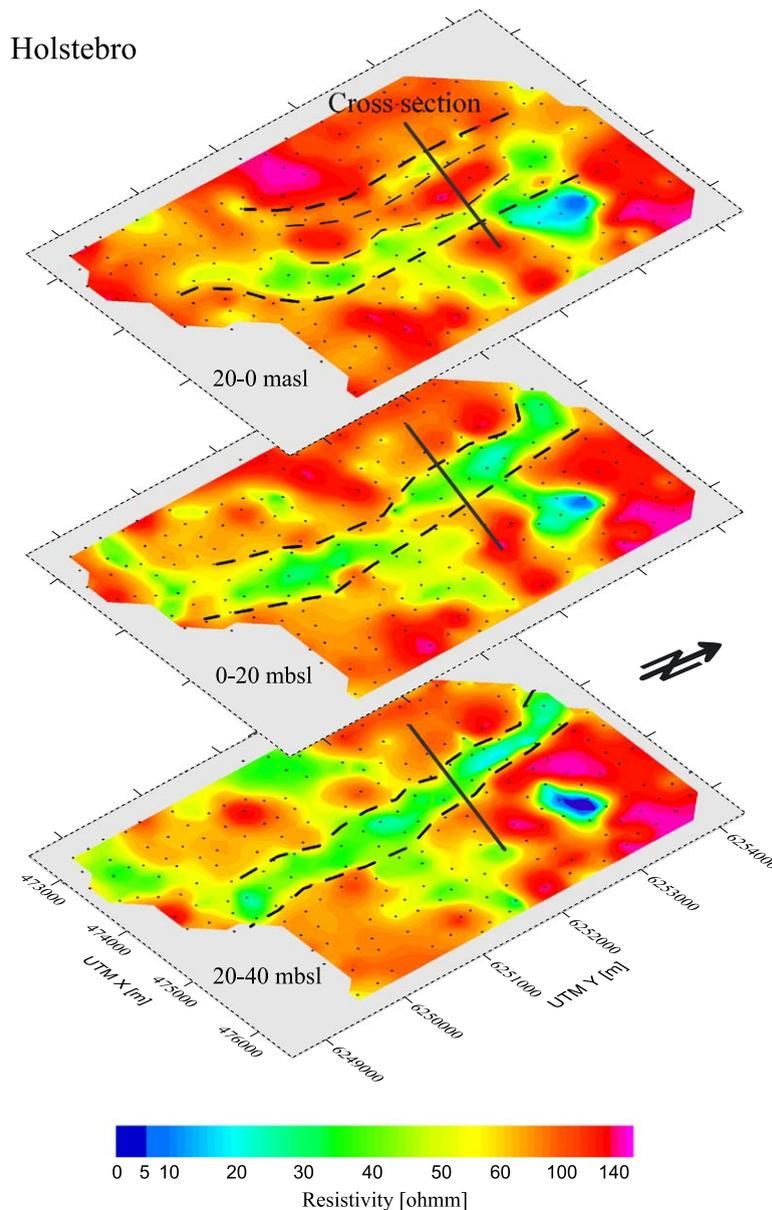
Fig. 4. The Holstebro buried valley depicted in contoured depth slices of 20 m mean resistivity intervals constructed from 1-D inverse models of 224 TEM soundings. Thick dashed lines mark valley boundaries. Thin dashed lines mark internal incision boundaries. The solid, black line marks the location of the cross-section model shown in Fig. 5. Field survey: Dansk Geofysik.
