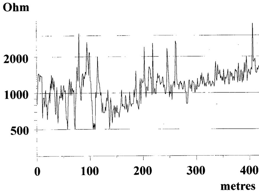
**Fig. 2.** The figure shows the resistance between the current electrodes as the tail is moved along the test profile. The soil is sandy moraine clay and the work was carried out on a sunny day. The resistance varies rapidly but within the limits of the current generator to be able to emit a constant current into the ground.
