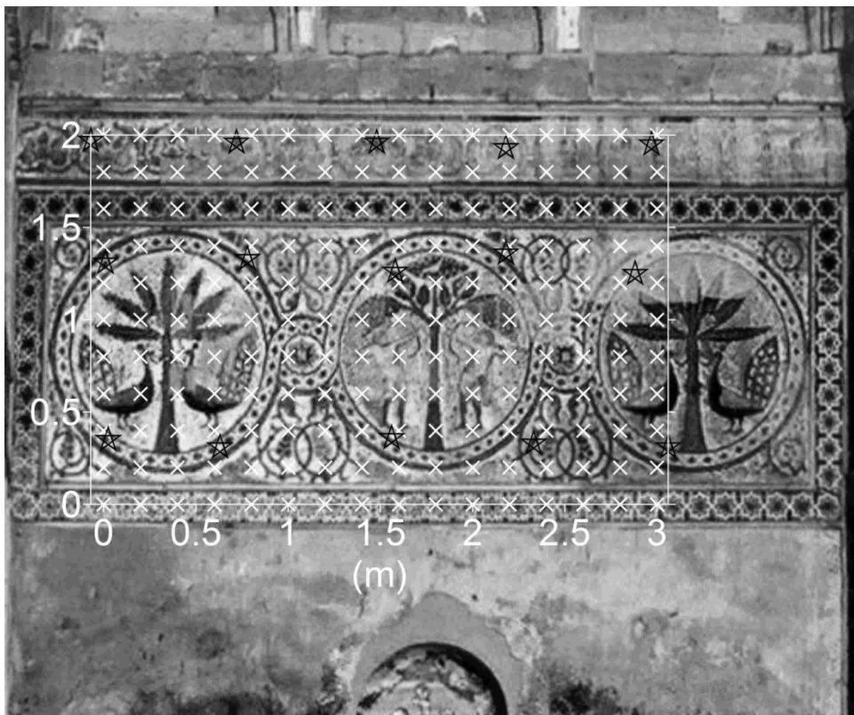
Figure 3. White crosses: potential electrodes; black stars: current electrodes.
