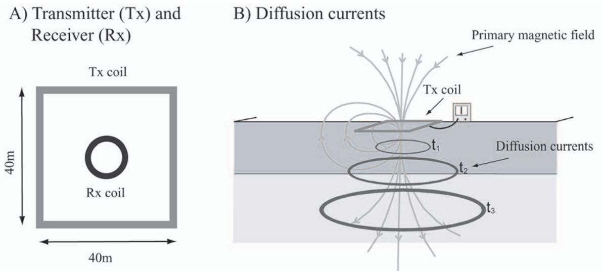
Fig. 3. A. Sketch of the TEM equipment setup. The transmitter (Tx) coil is typical  $40 \times 40 \text{ m}^2$ . The receiver (Rx) coil is located in the centre of the Tx. B. Physics of the TEM method in a schematic view. The induced currents in the ground are illustrated as loops at three successively increasing times.
