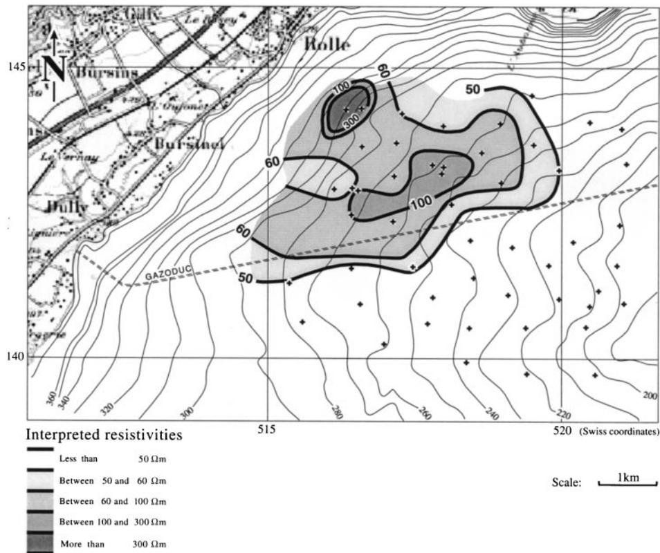
**Figure 10.** Interpreted iso-resistivity curves (in  $\Omega\text{m}$ ).
