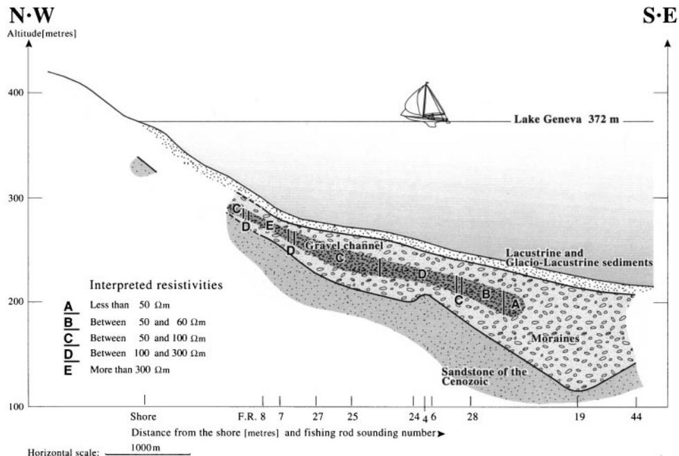
**Figure 11.** Cross-section offshore Rolle.
