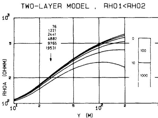
Fig. 4. Apparent resistivity curves for the six standard frequencies for a two-layer model of increasing type.
