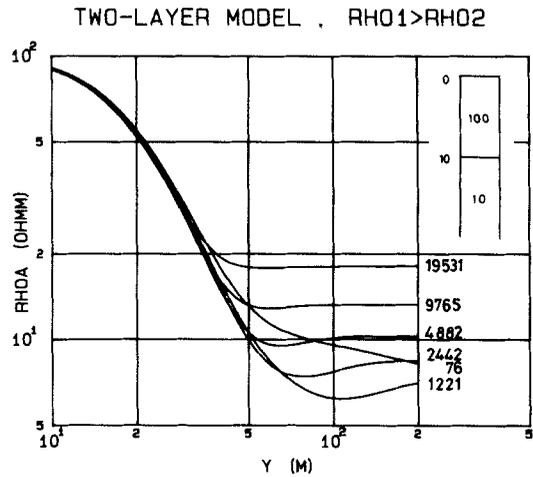
Fig. 5. Apparent resistivity curves for the six standard frequencies for a two-layer model of decreasing type.
