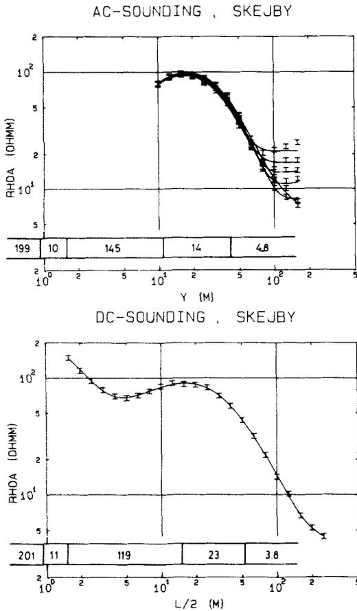
Fig. 7. An interpretation of an AC-geoelectrical sounding together with an interpretation of an ordinary DC-geoelectrical sounding in the Schlumberger configuration made at the same location in Skejby. Data for the AC-geoelectrical sounding have been recorded in the interval from 10 m to 200 m with a density of 10 per decade. The parameters of the topmost two layers of the AC model have been taken from the DC interpretation.
