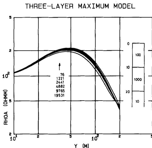
Fig. 6. Apparent resistivity curves for the six standard frequencies for a three-layer model of maximum type.
