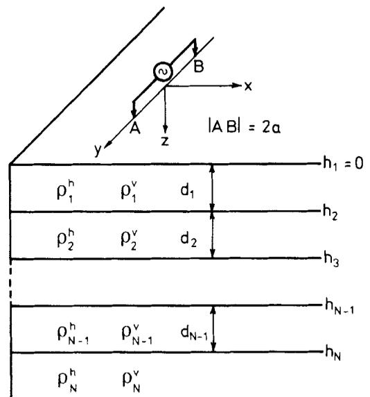
Fig. 1. The source and model configuration.  $\rho_i^h$ ,  $\rho_i^v$  and  $d_i$  are the horizontal resistivity, the vertical resistivity, and the layer thickness of the  $i$ 'th layer respectively.
