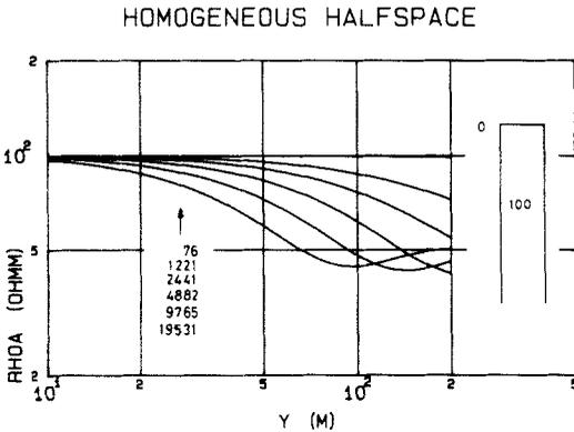
Fig. 3. Apparent resistivity curves for the six standard frequencies for a homogeneous halfspace.
