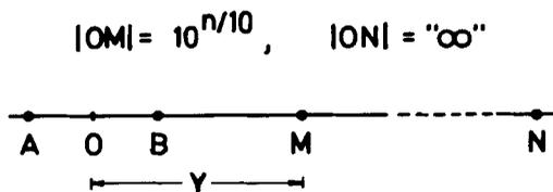
Fig. 2. The half-Schlumberger electrode configuration. A and B are current electrodes, M and N are potential electrodes.  $|OM| = Y$  is taken as the abscissa of the following model responses and data.
